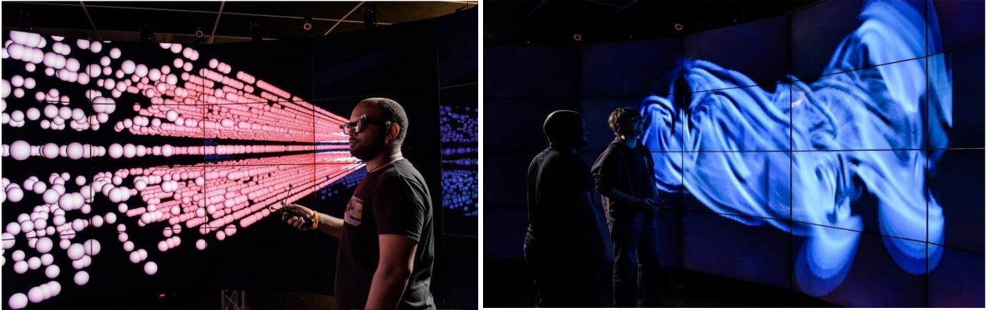
Figure 1 (left) shows point cloud rendering of the combustion dataset in CAVE2. Figure 2 (right) shows a volume rendering of a layer that is created when two fluids mix together in CAVE2.
